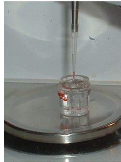
A precisely aspirated 1 uL sample in the disposable tip poised above the oil-filled cup on the scale. *One piston moving alone now blasts the sample into the oil* (several prior 1 uL blastoff globules can be seen). This setup produced the Blastoff data above.
