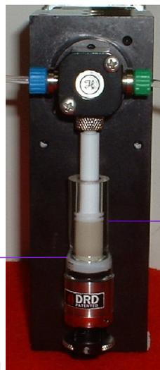
When the glass tube moves relative only to the hollow top Plunger Wiper Seal it gives the same ***high flow power as a 2.5 mL syringe.***
