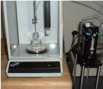
Probe tip underwater on scale during a repetitive 1 uL Differential aspiration study (standard up/down cycles, weights polled automatically when stable). This setup produced the aspiration data above.
