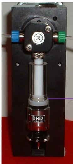
The cross-sectional area difference between the ID of the glass and the OD of the recessed spring-loaded bottom Piston is the same as a 100 uL syringe. When the glass tube moves relative to both the Plunger and the Piston simultaneously it gives the same ***fine resolution as a 100 uL syringe.***
