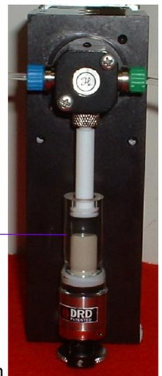
**DRS 20/300 INSTALLED IN HAMILTON PSD/4 PUMP MODULE**
